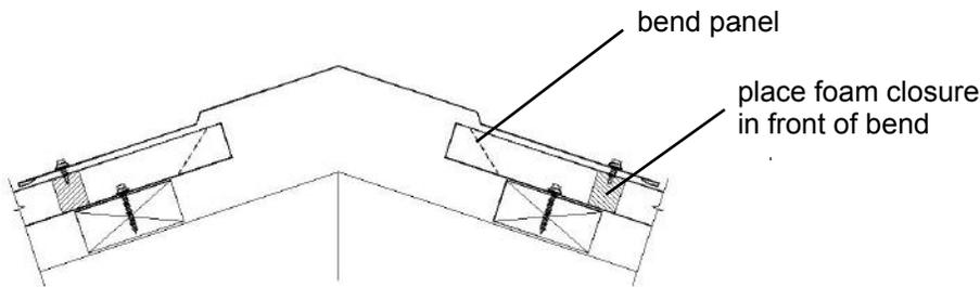
Notes: \*Turn Up Tool will bend roofing panels up to 24ga. thickness.
