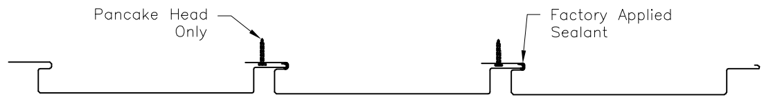
TYPICAL 1" REVEAL SEAM ENGAGEMENT
